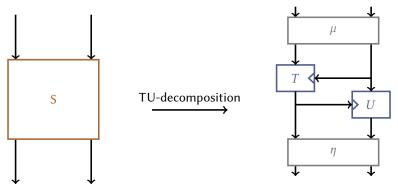
T and U are mini-block ciphers ;  $\mu$  and  $\eta$  are linear permutations.
